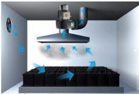
Example of a battery room (classified as zone 1), in which HYDROGEN is released: under these conditions, the use of extractor fans in the immediate vicinity of the batteries is compulsory and a further installation near the ceiling is also recoafication of these environments must be carried out by the relevant authorities.
